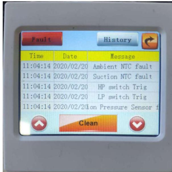
In most cases, system will automatically recover after troubleshooting. For some faults like low pressure protection, high pressure protection, discharge temperature protection,
